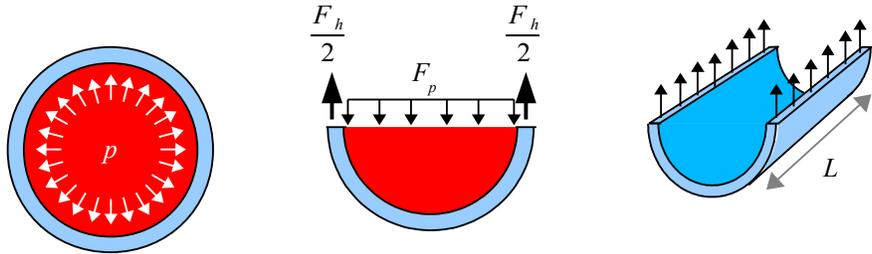
The fluid force and hoop force are equal. The hoop stress in the pipe wall is the hoop force divided by the wall thickness of the pipe times the length, times 2 walls:  $\sigma_h = \frac{F_h}{2tL} = \frac{F_p}{2tL} = \frac{p D_i L}{2tL} = \frac{p D_i}{2t}$ .
