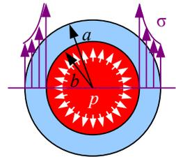
The stress at any given radius  $r$  is a function of the fluid pressure, the inside radius  $a$ , and the outside radius  $b$ . Stress
